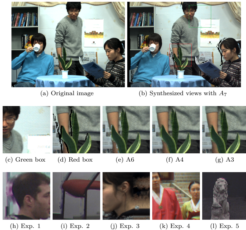
Figure 16.1 – Examples of non-uniform distortions in DIBR based synthesized views and examples of results of using different inpainting algorithms for dis-occluded regions filling.
