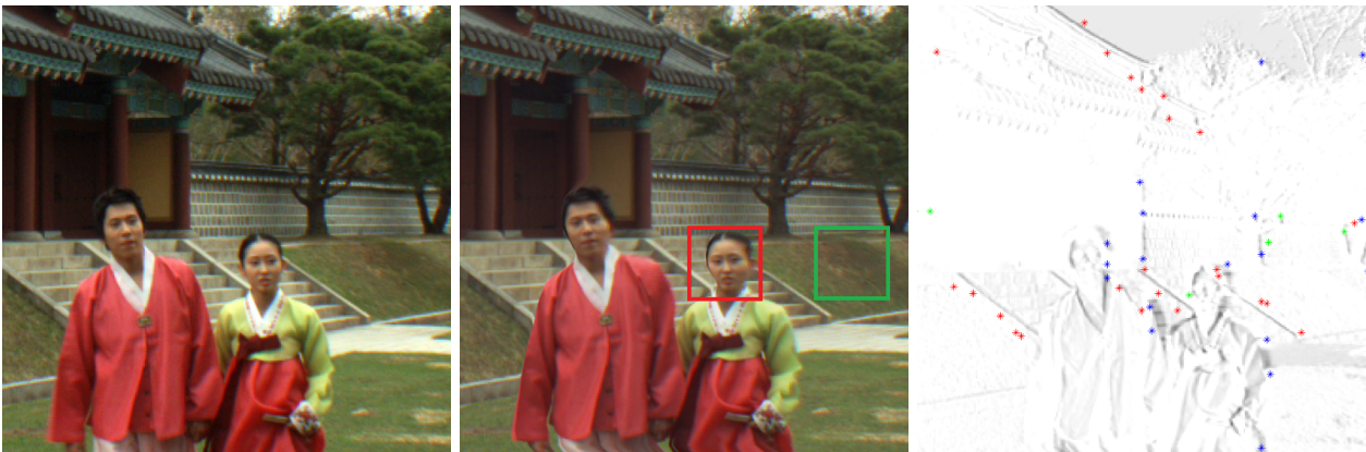
Figure 15.4 – Example of non-uniform distortion, Left: Reference, Middle: Synthesized view, Right: Error map
