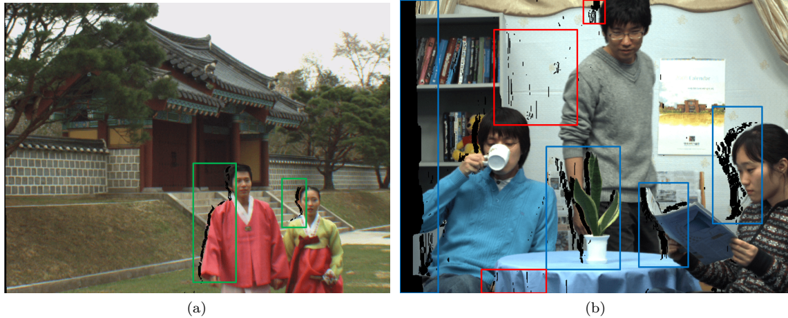
Figure 16.3 – Examples of typical dis-occluded regions introduced during the process of DIBR based views synthesis. (a) Examples of dis-occluded regions that are around foreground objects' boundaries (bounded by green boxes); (b) Examples of small and median size of dis-occluded regions (bounded by red and blue bounding boxes correspondingly) that distributed throughout the image;
