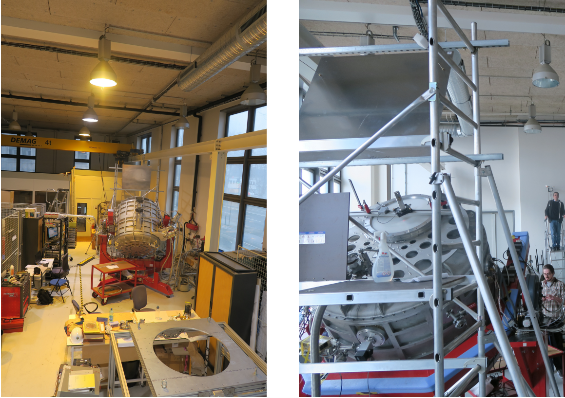
Figure 2. left: Photo of QUBIC looking along the line-of-sight from the calibration source. The reflection of the window is clearly visible in the flat mirror. right: The flat mirror is mounted on a scaffold at a height of 3.5 m and has a finely adjustable tilt angle using a system composed of a long screw.
