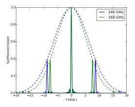
**Figure 2.** A cut of the QUBIC synthesized beam at two different frequencies showing how the location of the multiple peaks significantly changes for a small frequency change. This behaviour is at the basis of the spectro-imaging capabilities offered by bolometric interferometry. This figure can also be found in [27] from this series, dedicated to spectro-imaging.
