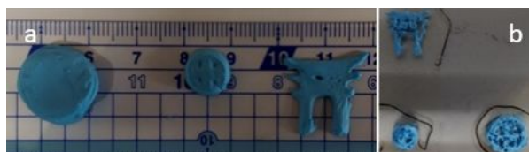
6 7 Figure 3. Photographs of CPL-1-based objects printed under the same conditions with inks 8 formulated with 35 wt% (a) and 51 wt% (b) of CPL-1.
