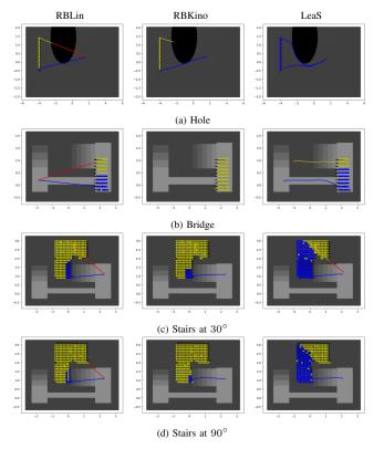
Fig. 5: Trajectories of steering methods with : valid trajectory to target (**Blue**), failed trajectory to target (**Yellow**), failed part of a trajectory (**Red**) and initial orientation (**Black Arrow**).
