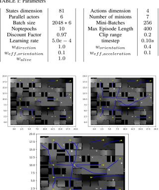
Fig. 3: Trajectories after 150K, 1M5 and 80M steps of learning on 10x10 grid training terrain with some initial positions and target directions (Yellow) and their trajectories (Blue).
