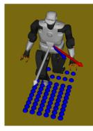
Fig. 2: Observable state with root orientation (white arrow), root velocity (Blue arrow), the desired target velocity and orientation (Red arrow) and the local height map (Blue dots).
