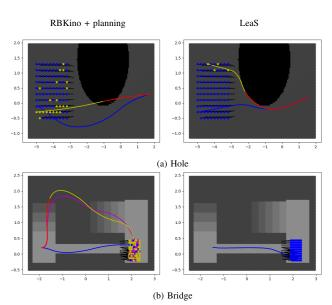
Fig. 6: Trajectories of RBKino with path planning and LeaS with : valid trajectory to target (**Blue**), failed trajectory to target (**Yellow**), failed part of trajectory (**Red**) and path valid but not optimal by not taking the bridge (**Magenta**).
