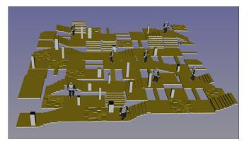
Fig. 1: The locomotion arena, a large stuctured simulation where our Talos agent learns in which direction to steer in order to generate stable contacts.
