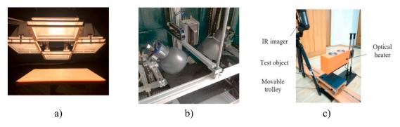
Fig. 2. Experimental IR thermographic setups with halogen lamps (a), Xenon flash tubes (b) and line-scanning implementation (c).
