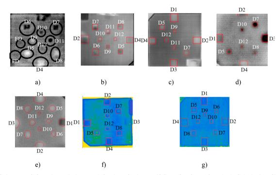
**Fig. 13.** Analyzing test results by Tanimoto criterion: a - optical stationary heating, one-sided procedure, front surface, TSR, 1st derivative (Fig. 3b), b - optical line-scanning heating, front surface (Fig. 4c), c - optical line-scanning heating, rear surface (Fig. 4d) d - flash heating, front surface, TSR, 1st derivative (Fig. 6b), e – flash heating, rear surface, TSR, 1st derivative (Fig. 6d), f - THz point-by-point scanning, Fig. 11a, g - THz line-scanning, Fig. 12.
