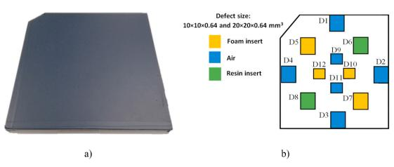
Fig. 1. Photo of black-painted test sample (a) and scheme of defects (b).
