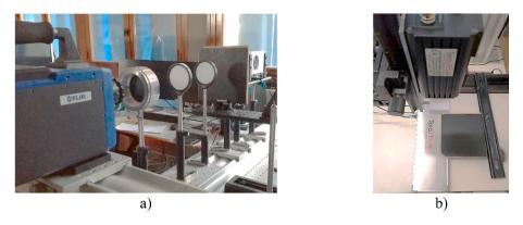
Fig. 9. Experimental setups for THz imaging in transmission mode: a – imaging scanning procedure, b – line-scanning procedure.
