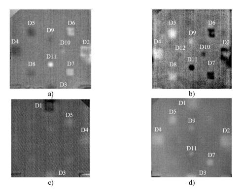
**Fig. 3.** Results of applying one- and two-sided test procedures (optical heating with 2 kW halogen lamps for 10 s (a–c) and 20 s (d): a – one-sided procedure, front surface (A), PCA image, 3rd component, b - one-sided procedure, front surface (A), TSR image, 1st derivative; c - one-sided procedure, rear surface (B), PCA image, 3rd component, d - two-sided procedure, front surface (A), PCA image, 1st component.
