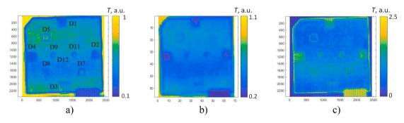
Fig. 11. Results of applying THz imaging scanning procedure in transmission mode: a - raw image, b - same as a), after  $5 \times 5$  spatial averaging, c - same as a), in logarithmic scale.
