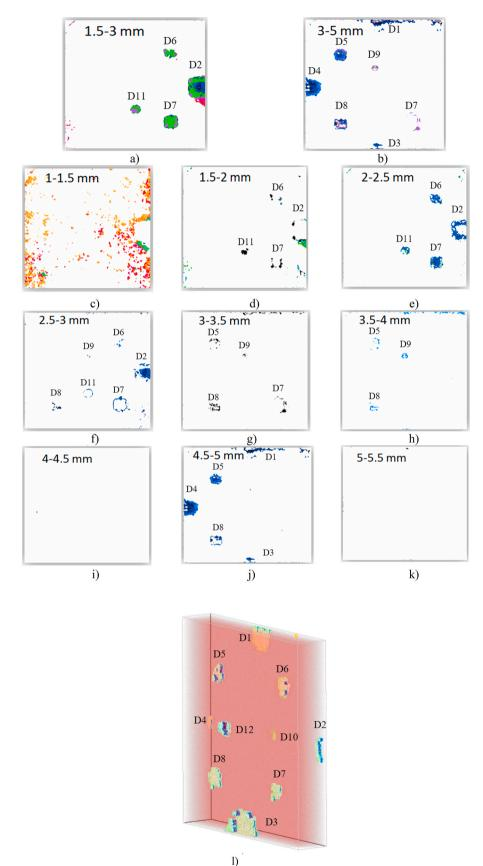
Fig. 8. Thermal tomography results: a – layer 1.5–3 mm, b – 3–5 mm, c – 1–1.5 mm, d – 1.5–2 mm, e – 2–2.5 mm, f – 2.5–3 mm, g – 3–3.5 mm, h – 3.5–4 mm, i – 4–4.5 mm, j – 4.5–5 mm, k – 5–6.5 mm, l – 3D reconstruction.
