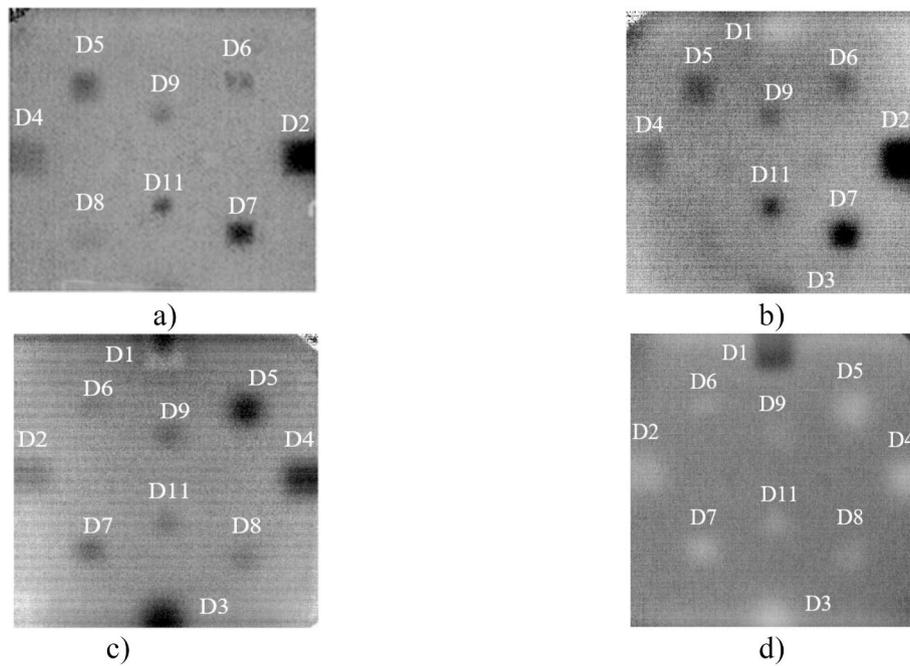
**Fig. 6.** Results obtained by using flash heating in one-sided (a, b) and two-sided (c, d) test procedures: a – front surface (A), PCA image, 1st component, b – front surface (A), TSR image, 1st derivative, c - rear surface (B), PCA image, 2nd component, d - rear surface (B), TSR image, 1st derivative.
