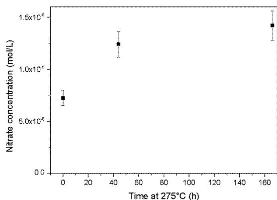
Fig. 8 Increases in the nitrate concentration during autoclave cleaning with an ammonium hydroxide solution at 275 °C
