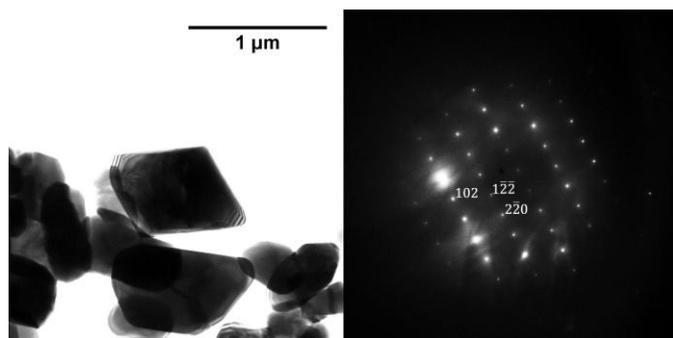
Fig. 6 TEM image of a hexagonal bipyramid crystal and power spectrum of image which serves to identify the crystal, zone axis  $[2\bar{2}1]$
