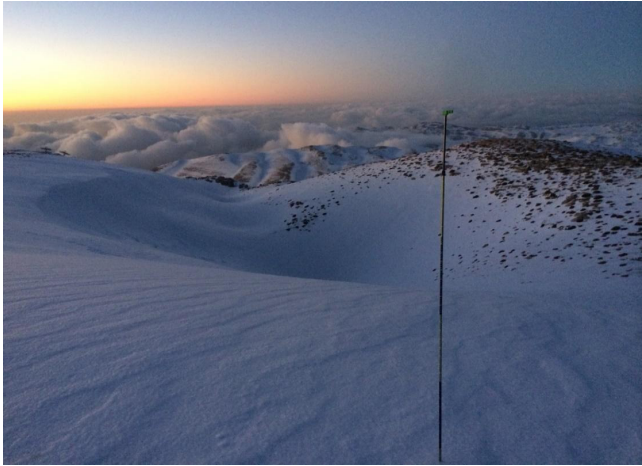
Figure 12. Snow redistribution following a major snowfall event at 2310 m a.s.l., 200 m away from the MZA AWS (located to the left of the image). Image taken on 15 January 2016. Snow depth at the station was 7.5 cm. Snow depth measured with snow probes in the vicinity ranged between 0 and 258 cm ( n = 46 ) with an average of 117 cm (median = 99 cm) and a standard deviation of 67 cm.
