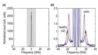
Figure 1: typical spectrum. (a) Raw spectrum where the contribution of Rayleigh scattering is indicated by the grey box. (b) Zoom-in on the Stokes (negative frequencies) and anti-Stokes (positive frequencies) peaks for a healthy tissue (black, intensity multiplied by 2 for clarity) and a caries lesion (blue line). Fits by Lorentzian functions are superimposed (red dashed lines).
