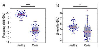
Figure 2: Comparison between healthy tissues (n=34) and caries lesions (n=39). Distributions of (a) frequency shift and (b) linewidth (\*\*\*\*p<0.0001, \*p<0.005, unpaired two-tailed t-test). The bottom and top edges of each grey box indicate the 25th and 75th percentiles, respectively. The red central line indicates the median. The whiskers extend to the most extreme data points not considering outliers ('+' symbol).
