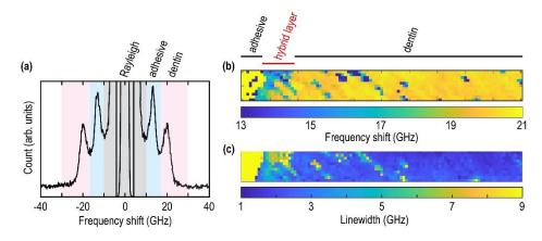
**Figure 9: imaging the hybrid layer.** (a) typical spectrum at the dentin-adhesive interface. The peaks arising from dentin and adhesive are shown in blue and pink, respectively. (a) Frequency shift and (b) linewidth maps of the hybrid layer.
