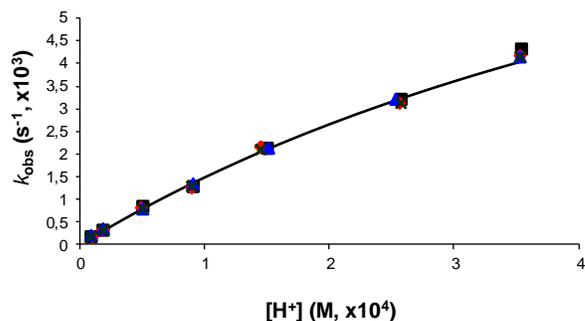
Figure 1. Dependence of the pseudo-first-order rate constants (*k*<sub>obs</sub>) on the concentration of H<sup>+</sup> and Cu(II) ions for the [Mn(PC2A-BP)] complex. The excess of the exchanging metal ion was ×10 (■), ×20 (◆), ×30 (▲) and ×40 (×) folds. The line corresponds to the best fit of the *k*<sub>obs</sub> values to eqn. 2.
