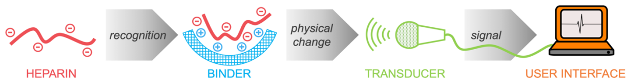
Figure 3. A schematic representation of a sensor for heparin.
