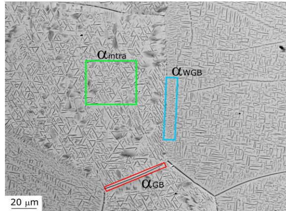
Figure 2: BSE image of the microstructure of the alloy prior deformation. The \alpha precipitates appear in dark in the \beta matrix.
