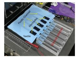
Figure 3. Biofuel cell with serially connected 5 stacks and modified fluidic channel.
