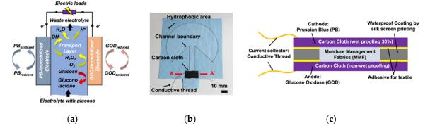
**Figure 1.** A single electrode biofuel cell: (**a**) working principle (**b**) fabricated biofuel cell (**c**) cross-section of AA' of the electrodes.
