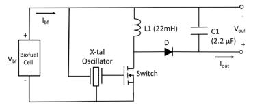
Figure 10. Schematic of biofuel cell energy harvester with power management circuit.
