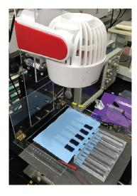
(a) Biofuel cell measurement setup
