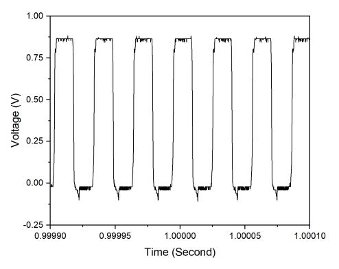
Figure 14. Output signal of oscillator.
