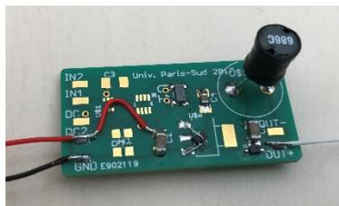
**(b)** Power management circuit board**Figure 13.** Measurement setup and power management board for biofuel cell with 5 electrodes.
