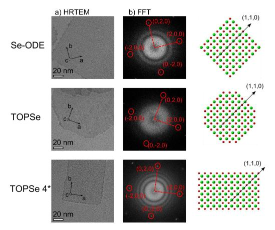
**Figure 4.** Facets control: from left to right, HRTEM images of the NPLs after unfolding and FFT on the HRTEM images. First row, nanosheets synthesized with Se-ODE, exhibiting only (110) facets. Second row, NSs synthesized using TOPSe exhibiting both (110) and (100) facets. Third row, NSs synthesized using TOPSe exhibiting only (100) facets. On the right, the corresponding model of the platelets with its folding axis has been represented.
