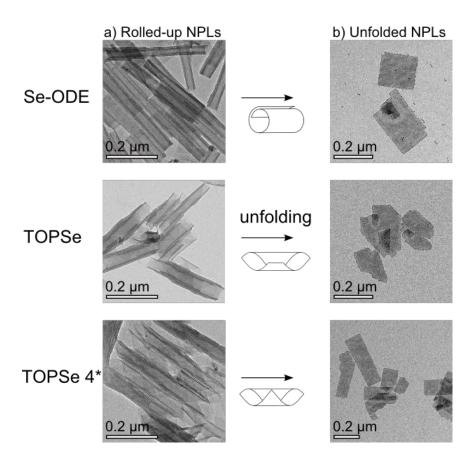
**Figure 3** Facets control: from left to right, TEM images after the synthesis, and after unfolding. First row, nanosheets synthesized with Se-ODE. Second row, NSs synthesized using TOPSe. Third row, NSs synthesized using TOPSe.
