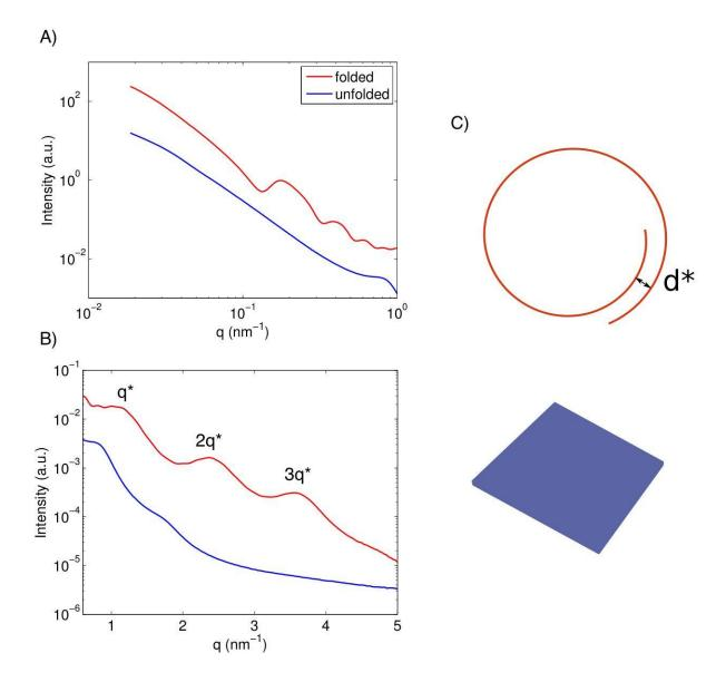
**Figure 2.** Small-Angle X-Ray Scattering: A) Low q scattering pattern for unfolded and folded nanoplatelets. B) High q scattering pattern for the same samples. C) Schematic representation of the structure of the nanoplatelets. The distance d\* corresponds to the broad Bragg peaks visible at high q values.
