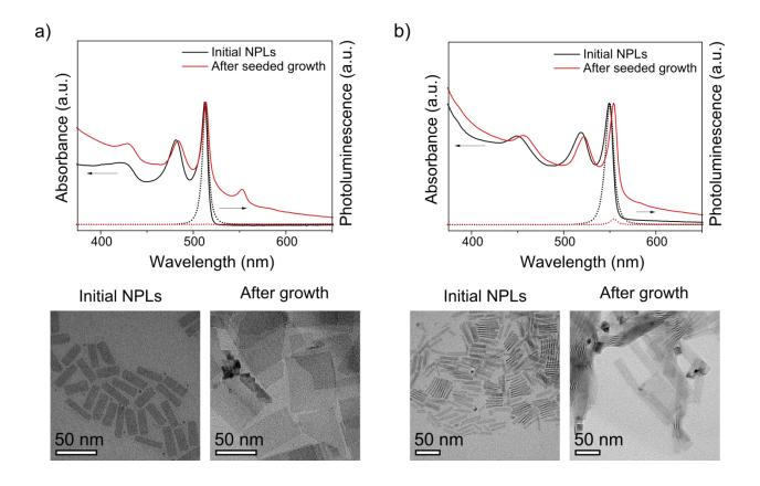
**Figure 5.** Lateral extension of a) 513 nanosheets and b) 553 nanosheets. Absorption and TEM images of the initial NPLs and the nanosheets after a continuous injection of precursors.
