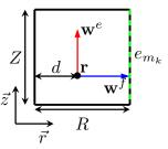
Figure 1. Axial-symmetric vector edge (red) and face (blue) shape functions related to edge  $e_{m_k}$ . An equivalent representation holds for edges along the r direction.
