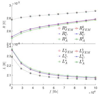
Figure 5.  $Z_{eq}$  of the induction cookware. Results obtained from A-code, C-code, and FEM for cases (a) and (b).
