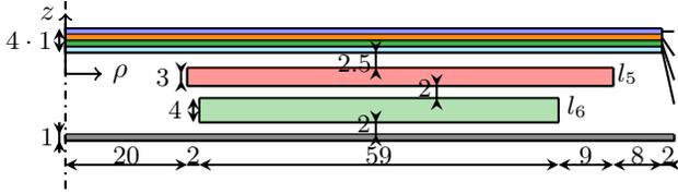
Figure 4. Axial-symmetric model of the induction cookware. Dimensions are in mm.  $l_1$ ) Stainless Steel,  $l_2$ ) Aluminum,  $l_3$ ) Magnetic Steel,  $l_4$ ) Stainless Steel,  $l_5$ ) External coil,  $l_6$ ) Ferrite (flux concentrator),  $l_7$ ) Aluminum (shield).
