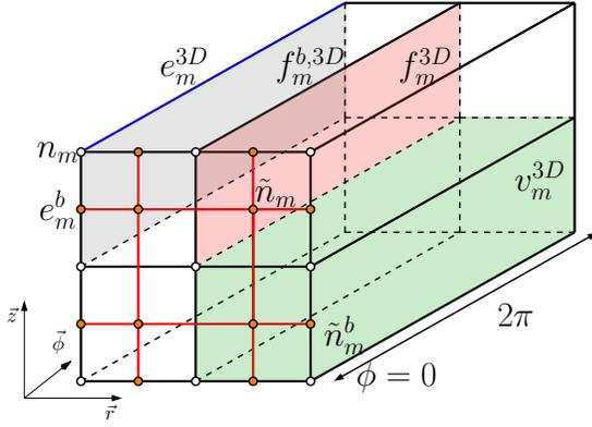
Figure 3. Primal and dual geometric entities of the magnetic grid for the coulombian formulation. Rectified axisymmetric geometry.
