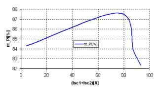
Fig.15. DC/DC converter efficiency
