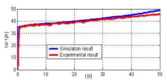
Fig.8: First supercapacitors module current
