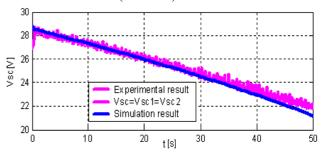
Fig.6: Two supercapacitors modules voltages
