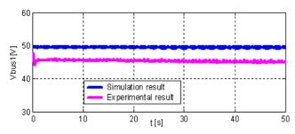
Fig.12: DC-bus voltage
