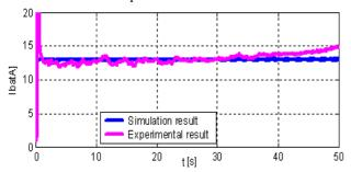
Fig.5: Battery current control results
