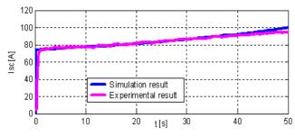
Fig.11: Supercapacitors modules full current
