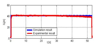
Fig.7: Hybrid vehicle DC-bus full current
