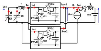
Fig.2: Parallel topology of the buck-boost converters
