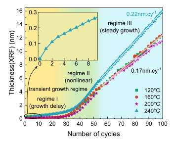
FIG. 1. Equivalent Thickness(XRF) of the deposited ZnO layers as a function of ALD cycle number for four different substrate temperatures:  $120^{\circ}$ C (green squares),  $160^{\circ}$ C (dark red circles),  $200^{\circ}$ C (purple stars), and  $240^{\circ}$ C (light blue triangles). Inset: Close-up of the Thickness(XRF) vs cycle number for the  $240^{\circ}$ C sample for cycles 0-9.
