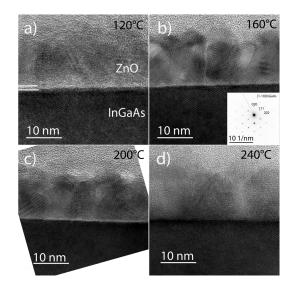
FIG. 6. Cross-sectional TEM images of samples grown at  $120^{\circ}$ C (a),  $160^{\circ}$ C (b),  $200^{\circ}$ C (c), and  $240^{\circ}$ C (d), after 100 ALD cycles. The inset in Figure (b) shows the InGaAs diffraction plane perpendicular to the  $[1\overline{10}]$  zone axis.
