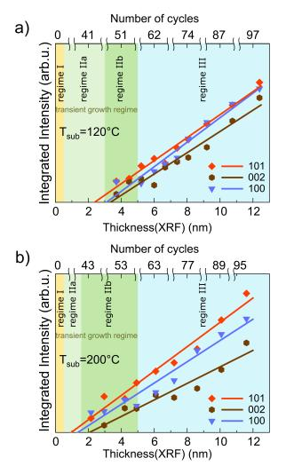
FIG. 5. The integrated **100**, **002**, and **101** diffraction peak intensities (symbols) as a function of the ZnO layer thickness (bottom x-axis) and cycle number (top x-axis) for samples grown at (a)  $120^{\circ}$ C and (b)  $200^{\circ}$ C. Also shown are linear fits to the data.
