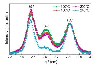
FIG. 4. The azimuth-integrated intensity profile obtained from in-plane zap-scan images as a function of  $q^{-1} = \left(\frac{2\sin\theta}{\lambda}\right)^{-1}$  for samples 120, 160, 200, and 240, measured after 100 ALD cycles. For comparison of the relative peak heights, all curves were normalized with respect to the intensity of the **100** diffraction peak.
