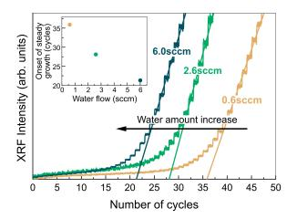
FIG. 2. XRF curves measured continuously during *in situ* ALD at the same substrate temperature of  $120^{\circ}$ C and for different water flows during the oxidant pulse: 0.6 sccm, 2.6 sccm, and 6.0 sccm. The straight line cross point with the cycle number axis gives a representative value of the onset of the steady-state growth. The value is reported in the inset as a function of water flow.
