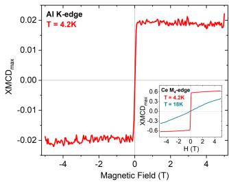
FIG. 3. Element-specific TFY XMCD intensity vs *H* measured at the Al *K* edge at E = 1560.5 eV for T = 4.2 K and at the Ce  $M_4$  edge at E = 891.5 eV for T = 4.2 K and T = 18 K (inset). Intensities are normalized to match those of the TFY XMCD spectrum at these energies.
