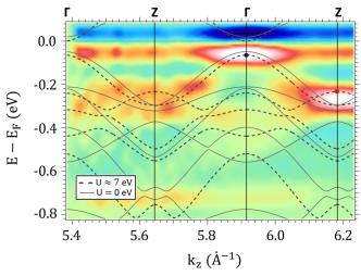
FIG. 10. Out-of-plane ARPES mapping over  $\Gamma Z$ , obtained by varying hv from 100 to 137 eV, and compared with DFT and DFT + U bands. The two dots refer to specific points of band 90 (located in  $\Gamma$  and Z, respectively) which are used in the text and also shown in Fig. 11. This band does not only exhibit a strong  $k_z$  dispersion, as demonstrated in this figure, but also crosses the Fermi level, as shown in Fig. 11.
