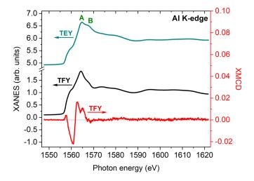
FIG. 2. Normalized TFY and TEY XANES spectra (left axis) along with the TFY XMCD spectrum (right axis, same scale as XANES) at the Al *K* edge, for T = 4.2 K and H = 1 T. The TFY XANES were corrected for self-absorption effects. Features of interest are labeled with capital letters and discussed in the text.
