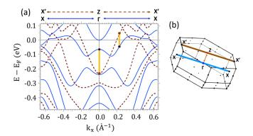
FIG. 11. (a) DFT + U band structure over  $\Gamma X$  and ZX', with the directions and the triclinic BZ of Mo<sub>4</sub>Ce<sub>4</sub>Al<sub>7</sub>C<sub>3</sub> given in (b). The effect of  $k_z$  broadening on band 90 is highlighted by the yellow lines, thus indicating a significant  $k_z$  delocalization of the conduction band.
