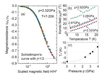
FIG. 7. Magnetoresistance measurements. (a) MR scaling in the Kondo regime for P = 2.32 GPa and T in the 7–20-K range, along with Schlottmann's theoretical MR for j = 1/2. (b) Kondo field vs temperature for various applied pressures (solid lines are linear fits to the data points). (c) Effective Kondo temperature vs applied pressure (solid line is a guide for the eyes).
