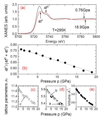
FIG. 5. Dependence of the Mo<sub>4</sub>Ce<sub>4</sub>Al<sub>7</sub>C<sub>3</sub> mixed valence on applied pressure. (a) Normalized XANES spectra measured at the Ce  $L_3$  edge for p = 0.76 GPa and p = 18.9 GPa, at T = 295 K. (b) Evolution of the valence with applied p. (c)–(d) Evolution of the lattice parameters with applied pressure. At 0.67 GPa  $\Delta c/c = 4.8 \times 10^{-2}$  and  $\Delta b/b = \Delta a/a = 3.8 \times 10^{-2}$ . (e) Evolution of unit cell volume with p.
