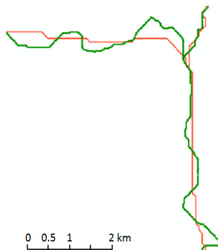
Figure 9. Detail of the hydrographic network extracted from SRTM (red) and Topodata (green). Source: [108].
