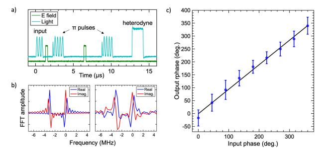
Figure 5: SEMM storage fidelity. (a) Photo-detector and voltage source signals for storage of a two-color pulse (3 MHz frequency difference). The heterodyne pulse detects the output echo. (b) Simulated (left) and experimental (right) Fourier transform of the heterodyne detected output echo for a two-color input pulse with a  $\pi/2$  relative phase shift. (c) Output vs. input phase shifts in two-color storage. Circles: experimental data, line: linear fit, correlation coefficient: 0.997.
