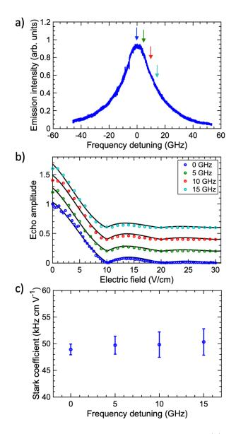
Figure 2: Optical frequency dependence of Stark coefficient. (a) Excitation spectrum of  $Eu^{3+}:Y_2O_3 \ ^7F_0 \rightarrow ^5D_0$  transition centered at 580.88 nm (vac.). (b) Normalized echo amplitude as a function of electric field at different excitation frequencies (arrows in (a)). Data are vertically translated for clarity. Solid lines are fits to Eq. 4. (c) Fitted Stark coefficient as a function of optical frequency from line center.
