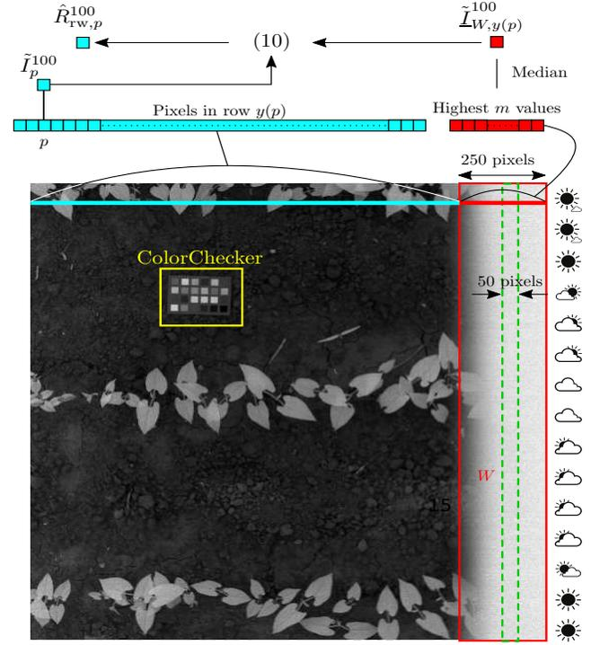
Fig. 3: rw-based reflectance estimation ( $k = 100$ ,  $\lambda^{100} = 780\text{nm}$ ).
