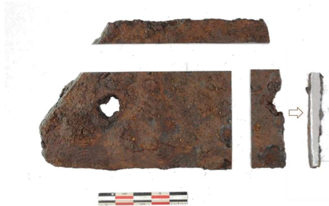
Figure 2 Archaeologic sample (CL13286) after being cut, and its cross section.
