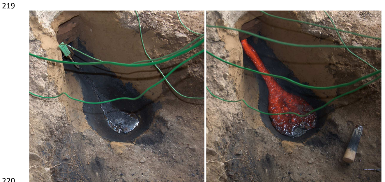
220 221 Figure 6, Running lead then slag from test STI- 8 222
