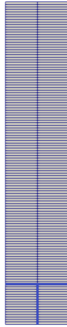
Figure 11: Discrete Fracture Model with the fracture network in bold and its uniform Cartesian mesh of size 2 \times 128 .
