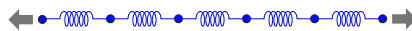
Figure 1: A chain of particles connected in series by breakable springs and loaded in tension.
