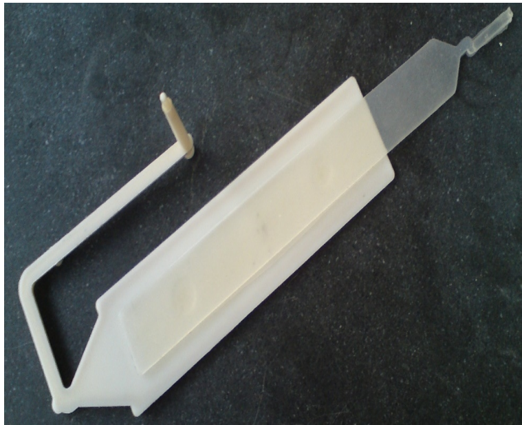
Figure 8. Over-mould of the PA66/LSR4350 peel test specimen.
