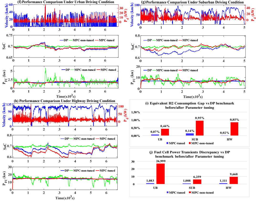
Fig.7 (f)-(j). EMS performance comparison before/after MPC penalty factor tuning: (f) performance comparison under urban driving condition; (g) performance comparison under suburban driving condition; (h) performance comparison under highway driving condition; (i) fuel economy discrepancy vs. DP benchmark; (j) fuel cell power transients discrepancy vs. DP benchmark.
