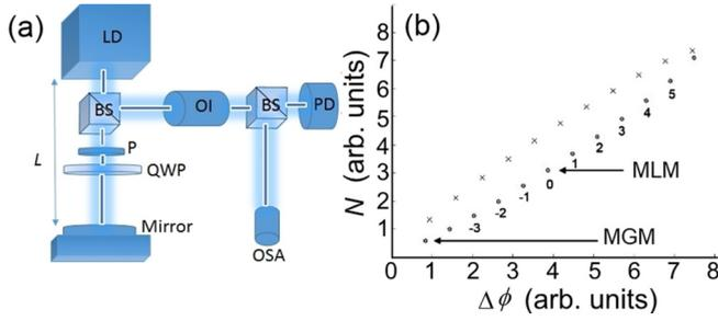
FIG. 1. (Color online) (a) Experimental setup. LD, laser diode; BS, beam splitter; PD, photodetector; P, polarizer; QWP, quarter-wave plate; OI, optical isolator; OSA, optical spectrum analyzer; and  $L$ , external-cavity length. LD is an intrinsically single-longitudinal mode InGaAsP DFB laser at 1550 nm with maximum power of 15 mW. (b) Ellipse structure of fixed points in  $\Delta\phi$ -vs- $N$  plane. Circles represent ECMs; crosses represent antimodes. Labels indicate mode number.
