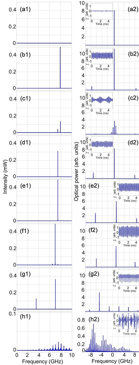
FIG. 3. (Color online) Experimental RF spectra (first column), and optical spectrum with OSA of  $\mathcal{I}(t)$  (second column), and associated  $\mathcal{I}(t)$  (inset): (a1) and (a2)  $\eta = 0.05$ , (b1) and (b2) 0.13, (c1) and (c2) 0.2, (d1) and (d2) 0.26, (e1) and (e2) 0.28, (f1) and (f2) 0.35, (g1) and (g2) 0.5, and (h1) and (h2) 0.8.
