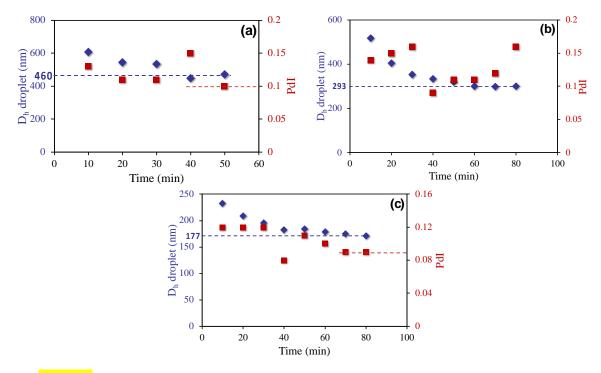
**Figure 3.** Evolution of droplet diameter as a function of time for styrene miniemulsions prepared using the ultra-turrax (rotational speed at 20,000 rpm) as emulsification device and hexadecane (HD) as the hydrophobe. (**a**) 1.5 wt.% of SDS (**b**) 3 wt% of SDS, and (**c**) 3 wt% of in situ generated K-oleate.
