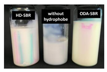
**Figure 7.** Macroscopic aspects of the SBR latexes synthesized based on the recipe in Table 2, using HD or ODA as the hydrophobe or without hydrophobe.
