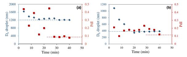
**Figure 2.** Progress of dynamic light scattering (DLS) droplet diameter over time for styrene miniemulsions obtained using the rotor–stator mixer operating at a rotational speed of 3000 rpm with different surfactants: (a) 1.5 wt% of SDS and (b) 1.5 wt% of in situ generated K-oleate, using HD as the hydrophobe.
