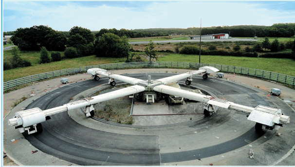
Figure 2: Fatigue carousel at IFSTTAR [11]
