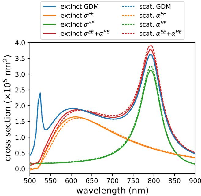
FIG. 11. Extinction (solid lines) and scattering (dashed lines) cross sections of a dielectric sphere (constant and real refractive index  $n = 4$ ) with radius  $r = 100$  nm, placed in vacuum and illuminated by a linear polarized plane wave. The sharp resonance around 525 nm can be attributed to a quadrupole mode.
