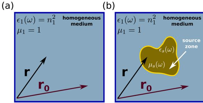
FIG. 1. Sketch used to implement the concept of generalized electromagnetic propagator. (a) Transparent reference medium with  $\epsilon_1(\omega) = n_1^2$  and  $\mu_1 = 1$ , and (b) material system of arbitrary shape, also called the *source zone*, embedded in the reference medium [permittivity  $\epsilon_s(\omega)$  and permeability  $\mu_s(\omega)$ ].
