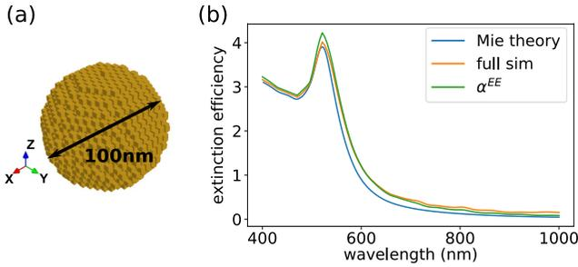
FIG. 7. Extinction efficiency spectra computed for a gold sphere of diameter  $D = 100$  nm using Mie theory (blue curve), the full GDM simulation (orange curve) and the effective polarizability approximation (green curve). The sphere is placed in vacuum and illuminated by a linear polarized plane wave.
