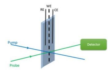
*Figure 17. Electrochemical cell for transient absorption spectroelectrochemistry measurements.*
