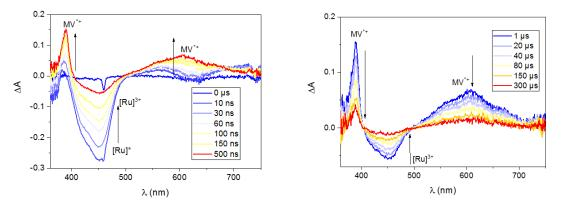
Figure 18. Transient spectra at indicated delay times generated by 460 nm laser excitation of  $[Ru(bpy)_3]^{2+}$  (35  $\mu$ M) and  $MV^{2+}$  (10 mM) in Ar-saturated water.
