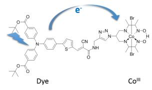
*Figure 26. Structure of a dye-cobalt catalyst studied by transient absorption spectroelectrochemistry [69].*
