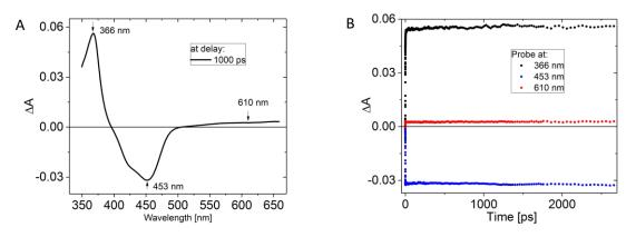
Figure 11. (A) UV-vis  $\Delta A$  spectrum recorded for a solution of  $[Ru(bpy)_3]^{2+}$  in water after excitation at 446 nm. (B) Selected  $\Delta A$  kinetic traces at the probe wavelengths of 366, 453 and 610 nm.
