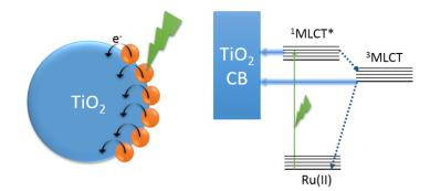
Figure 20. Illustration of excitation of Ru(II)-polypyridyl dye sensitized TiO<sub>2</sub> and electron injection to the CB of TiO<sub>2</sub> following MLCT excitation of Ru(II) chromophore.
