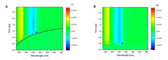
Figure 13. (A) GVD measured for a water solution of  $[Ru(bpy)_3]^{2+}$ , upon excitation at 410 nm in a 2-mm optical path sample cell. A dispersion of 1.4 ps of the time zero is observed in the 330-660 nm spectral range. (B)  $\Delta A$  spectra after GVD correction.
