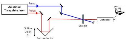
Figure 4. Basic principle of femtosecond transient absorption.
