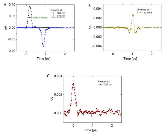
Figure 14. ΔA kinetics traces measured in pure water. A) Stimulated Raman scattering at 359 and 474 nm due to the O-H vibrations of water upon excitation at 410 nm. The full width at half maximum (FWHM) corresponds to the IRF (180 fs). B) Cross-phase modulation of the probe at 523 nm upon excitation at 410 nm. C) Two-photon absorption signal resulting from of the simultaneous absorption of pump and probe photons at 286 and 337 nm, respectively.
