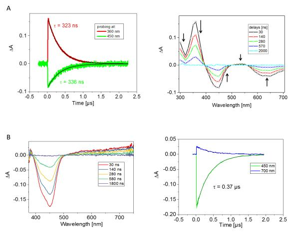
Figure 7. Transient absorption kinetics and spectra of the triplet state of  $[Ru(bpy)_3]^{2+}$  in water obtained using single wavelength measurements (A) and broadband measurements (B). In case (A) kinetics are measured in real-time by PMT coupled to a digital oscilloscope, and the transient spectra are calculated by data processing. In case (B) transient spectra at selected delay are measured by ICCD camera, and the kinetics can be calculated.
