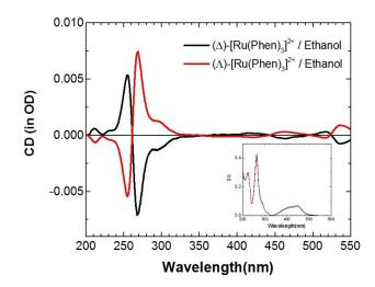
Figure 27. CD spectra of the two enantiomers of [Ru(phen)<sub>3</sub>]<sup>2+</sup> measured in ethanol with a home-made spectropolarimeter in our laboratories. Insert: Corresponding absorption spectra.
