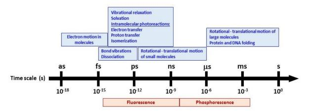
*Figure 2. Typical time scales of photophysical and photochemical processes occurring in solution.*
