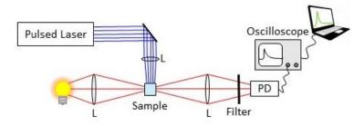
Figure 3. Basic principle of nanosecond-millisecond flash photolysis.
