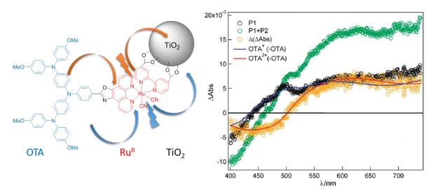
Figure 22. Structure of OTA-Ru<sup>II</sup>-TiO<sub>2</sub> and transient absorption spectra measured directly after single pulse (P1) and double pulse (P1+P2) 480 nm excitation. The orange curve indicates the difference spectrum between the double pulse and single pulse spectra. The blue and the red curves represent the differential spectra of OTA<sup>+</sup> and OTA<sup>2+</sup> obtained from spectroelectrochemistry. Reproduced from Ref. [42] by permission of American Chemical Society.
