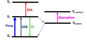
Figure 5. Three-state population model illustrating the formation of a transient nonemissive product in the singlet ground state from S<sub>1</sub>.
