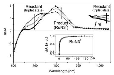
Figure 21. Transient absorption spectra observed by 530 nm laser excitation of RuN3sensitized TiO₂ film at time delay of 0.5 (■), 10 (○) and 150 ps (▲) pump-probe delay. Inset: Time profile at 860 nm corresponding to RuN3 cation. The figure was published in Ref. [19] and reproduced by permission of the American Chemical Society.
