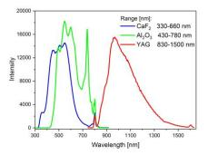
Figure 9. White light continua obtained by focusing ~100 fs laser pulses ( $\lambda$  = 800 nm) in a selection of media: CaF<sub>2</sub>, Al<sub>2</sub>O<sub>3</sub> or YAG crystal.
