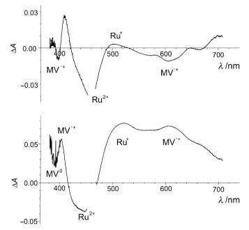
Figure 25. Transient spectra of  $[Ru(bpy)_3]^{2+}$ - $MV^+$  at 3 ps (top) and  $[Ru(bpy)_3]^{2+}$ - $MV^0$  at 5 ps (bottom) after 460 nm laser excitation. Reproduced from Ref. [68] by permission of John Wiley and Sons.
