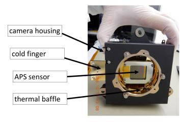
**Fig. 20.** Focal Plane Array with APS sensor and cold finger during assembly. The optical baffle in front of the detector is not yet mounted, such that the gold plated thermal baffling can be seen.
