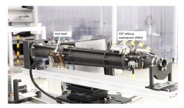
Fig. 11. FDT tube with PMP included.
