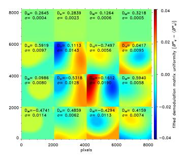
**Fig. 41.** 2D fitted demodulation matrix for the HRT and a PMP temperature set point of 40 °C. Each subimage shows the variation of one matrix element across the entire 2048 × 2048 pixels area of the HRT FOV. The mean value of each matrix element,  $\langle D_{ij} \rangle$ , is subtracted and annotated (together with the standard deviation,  $\sigma_{ij}$ , across the FOV within the illuminated area) to each element.
