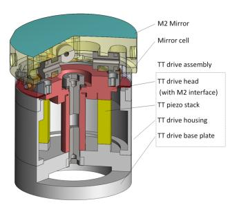
$\textbf{Fig. 23.} \ \ \textbf{Schematic overview of the tip/tilt drive assembly with mounted} \ \ \textbf{M2 mirror}$
