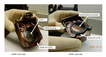
Fig. 17. Polarisation State Analyser of the HRT path.
