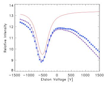
**Fig. 37.** Spectral scans across the Fe<sub>1</sub>6173 Å spectral line (crosses and asterisks) obtained from different sectors of the science detector during HRT ground calibration. The solid line denotes a convolution of the FTS spectrum with an Airy function of 106 mÅ FWHM.
