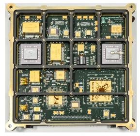
Fig. 32. Flight model of the Data Processing Unit.
