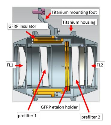
Fig. 18. Optomechanical arrangement of the Filtergraph.
