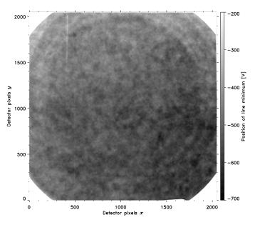
**Fig. 38.** Etalon cavity map obtained from Gaussian fits to the centre of the Fe 16173 Å spectral line during HRT ground calibration. The large-scale trend and the slight shift of the two scans shown in Fig. 37 arise from the solar rotation pattern imprinted in the incoming light, since the HRT FOV covers almost the entire solar disc at 1 AU distance, even if the feed optics does not provide a focused solar image.
