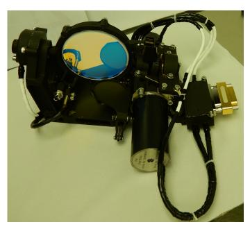
Fig. 13. SO/PHI Feed-Select Mechanism flight model.
