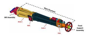
**Fig. 12.** Mechanical design of the FDT assembly. The FDT assembly is mechanically composed of three elements: the Front Support Assembly, the Main Structure and the M5 assembly. The Main Structure includes the FRM, the PMP, body 1 and body 2.
