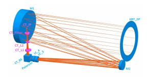
**Fig. 21.** Optical scheme of the ISS path. M2 is used as the tip/tilt compensator; CT\_BS is the beam splitter which feeds a small fraction of the light to the image plane (CT\_IP) in the Correlation Tracker Camera.
