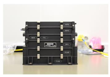
**Fig. 30.** Flight model of the E-Unit. The various subsystems are labeled. From top to bottom we have the high-voltage power supply; the analog, motor, and heater driver; the mezzanine memory board of the data processing unit and the tip-tilt controller; the main data processing unit board; the redundant power converter module; and the main power converter module.
