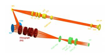
Fig. 10. Optical scheme of the FDT path.
