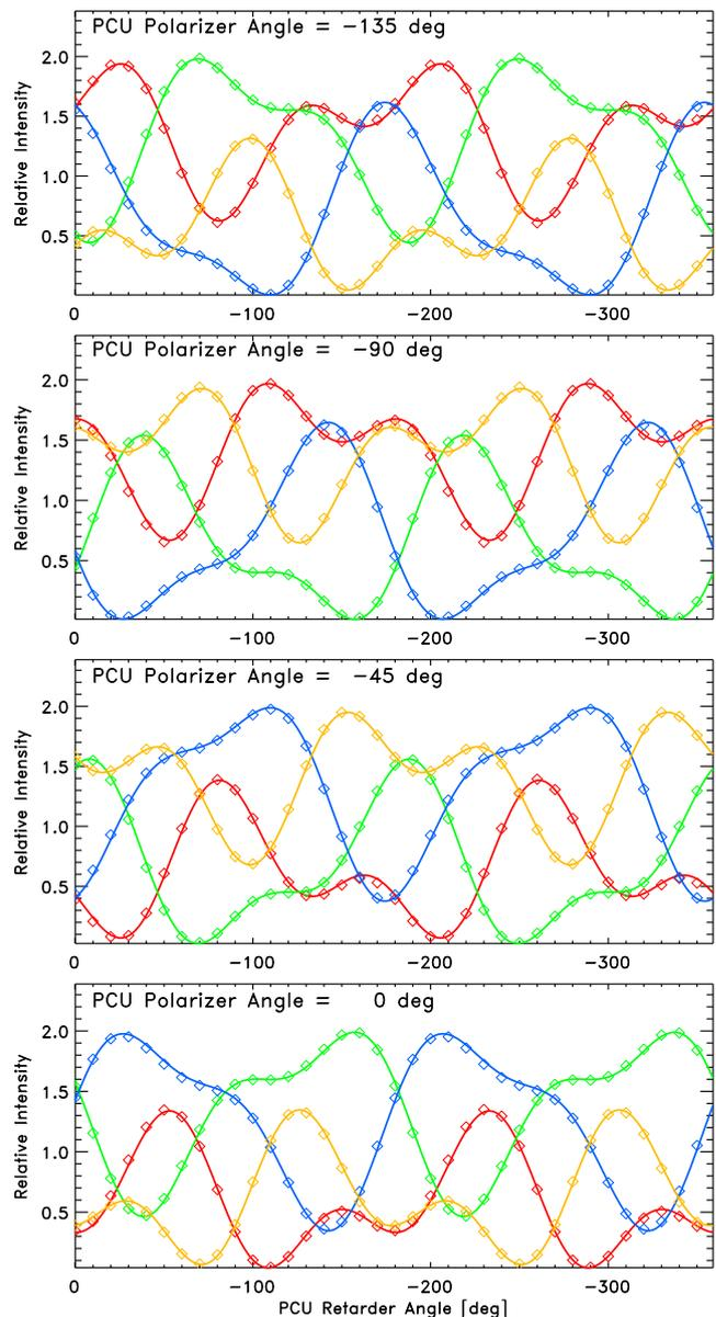
**Fig. 36.** Polarimetric calibration of the FDT for 45 °C liquid crystal temperature. The diamonds denote mean intensities of the images taken at the 4 polarimetric states of the SO/PHI modulation scheme (see Tab. 5) at each input polarimetric state; solid lines represent the fitted model.
