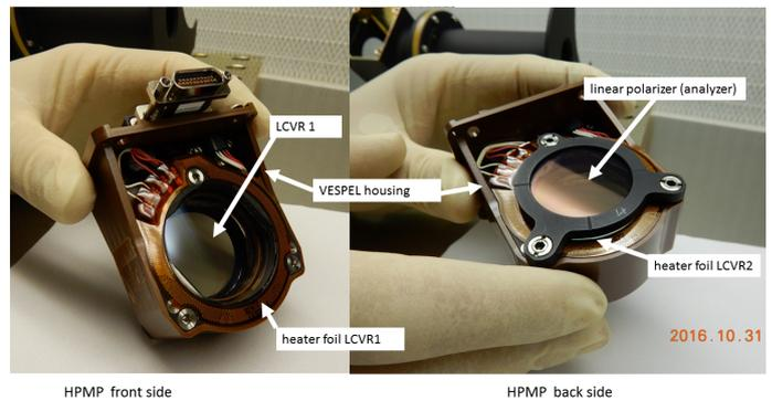
**Fig. 17.** Polarisation State Analyser of the HRT path.
