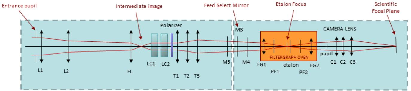
**Fig. 9.** Optics Block Diagram of the Full Disc Telescope path. L1 and L2 are lens1 and lens 2; FL is the field lens; LC1 and LC2 are the liquid crystal cells; T1, T2 and T3 are the triplet lenses 1, 2 and 3 respectively; M5, M3 and M4 are the folding mirrors; the Filtergraph oven includes the two lenses FG1 and FG2, the two components of the prefilter (PF1 and PF2) and the etalon; finally, the camera lenses (C1, C2 and C3) provide the image at the scientific focal plane.
