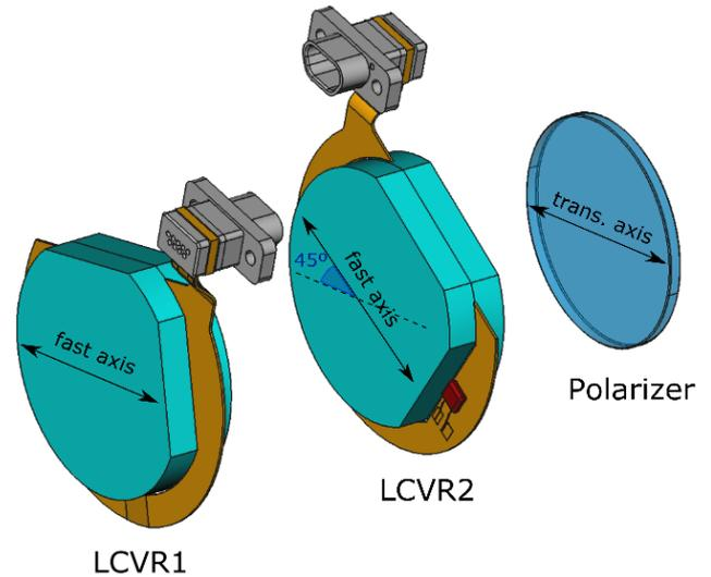
**Fig. 16.** Scheme of the Polarisation State Analyser.
