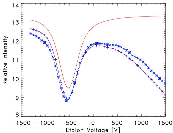
**Fig. 37.** Spectral scans across the Fe I 6173 Å spectral line (crosses and asterisks) obtained from different sectors of the science detector during HRT ground calibration. The solid line denotes a convolution of the FTS spectrum with an Airy function of 106 mÅ FWHM.
