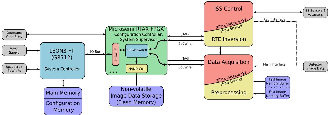
Fig. 31. Block diagram of the Data Processing Unit
