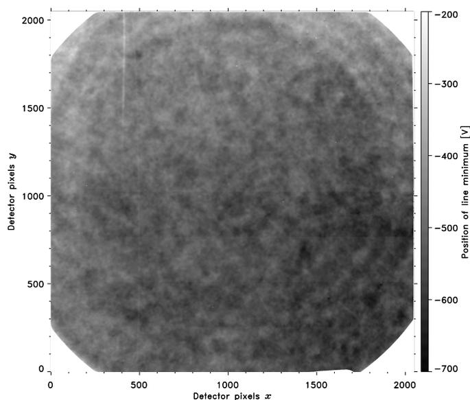
**Fig. 38.** Etalon cavity map obtained from Gaussian fits to the centre of the Fe I 6173 Å spectral line during HRT ground calibration. The large-scale trend and the slight shift of the two scans shown in Fig. 37 arise from the solar rotation pattern imprinted in the incoming light, since the HRT FOV covers almost the entire solar disc at 1 AU distance, even if the feed optics does not provide a focused solar image.
