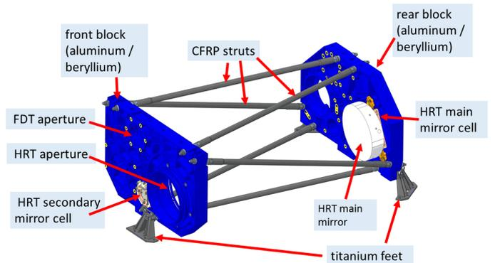
**Fig. 8.** HRT main structure, based on two end blocks and six CFRP struts.
