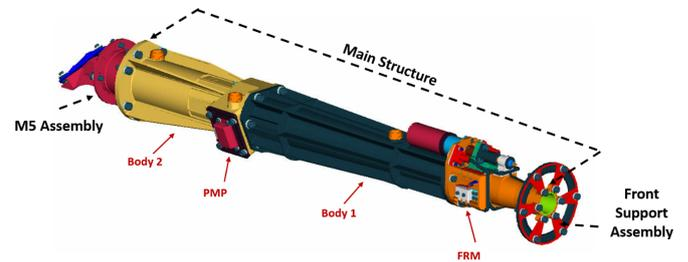
**Fig. 12.** Mechanical design of the FDT assembly. The FDT assembly is mechanically composed of three elements: the Front Support Assembly, the Main Structure and the M5 assembly. The Main Structure includes the FRM, the PMP, body 1 and body 2.
