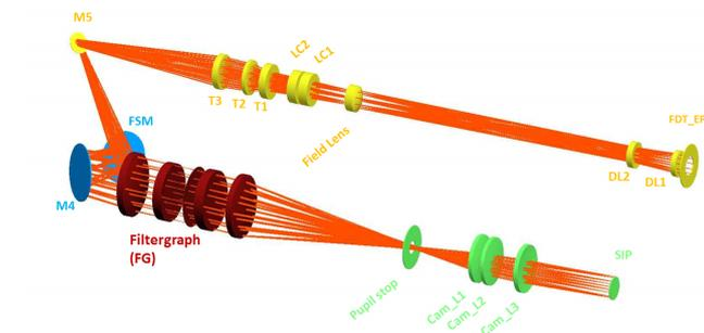
**Fig. 10.** Optical scheme of the FDT path.
