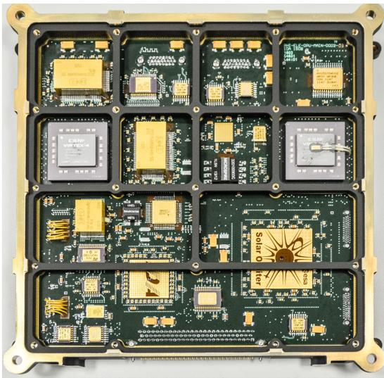
Fig. 32. Flight model of the Data Processing Unit.
