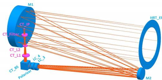
**Fig. 21.** Optical scheme of the ISS path. M2 is used as the tip/tilt compensator; CT\_BS is the beam splitter which feeds a small fraction of the light to the image plane (CT\_IP) in the Correlation Tracker Camera.
