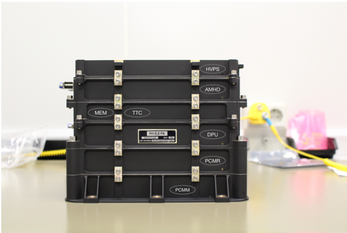
Fig. 30. Flight model of the E-Unit. The various subsystems are labelled. From top to bottom we have the high-voltage power supply; the Analogue, Motor, and Heater Driver; the mezzanine memory board of the data processing unit and the tip-tilt controller; the main data processing unit board; the redundant power converter module; and the main power converter module.
