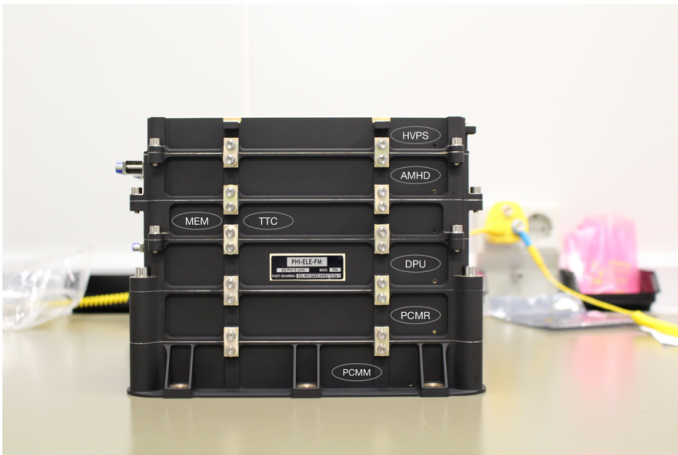
Fig. 30. Flight model of the E-Unit. The various subsystems are labeled. From top to bottom we have the high-voltage power supply; the analog, motor, and heater driver; the mezzanine memory board of the data processing unit and the tip-tilt controller; the main data processing unit board; the redundant power converter module; and the main power converter module.
