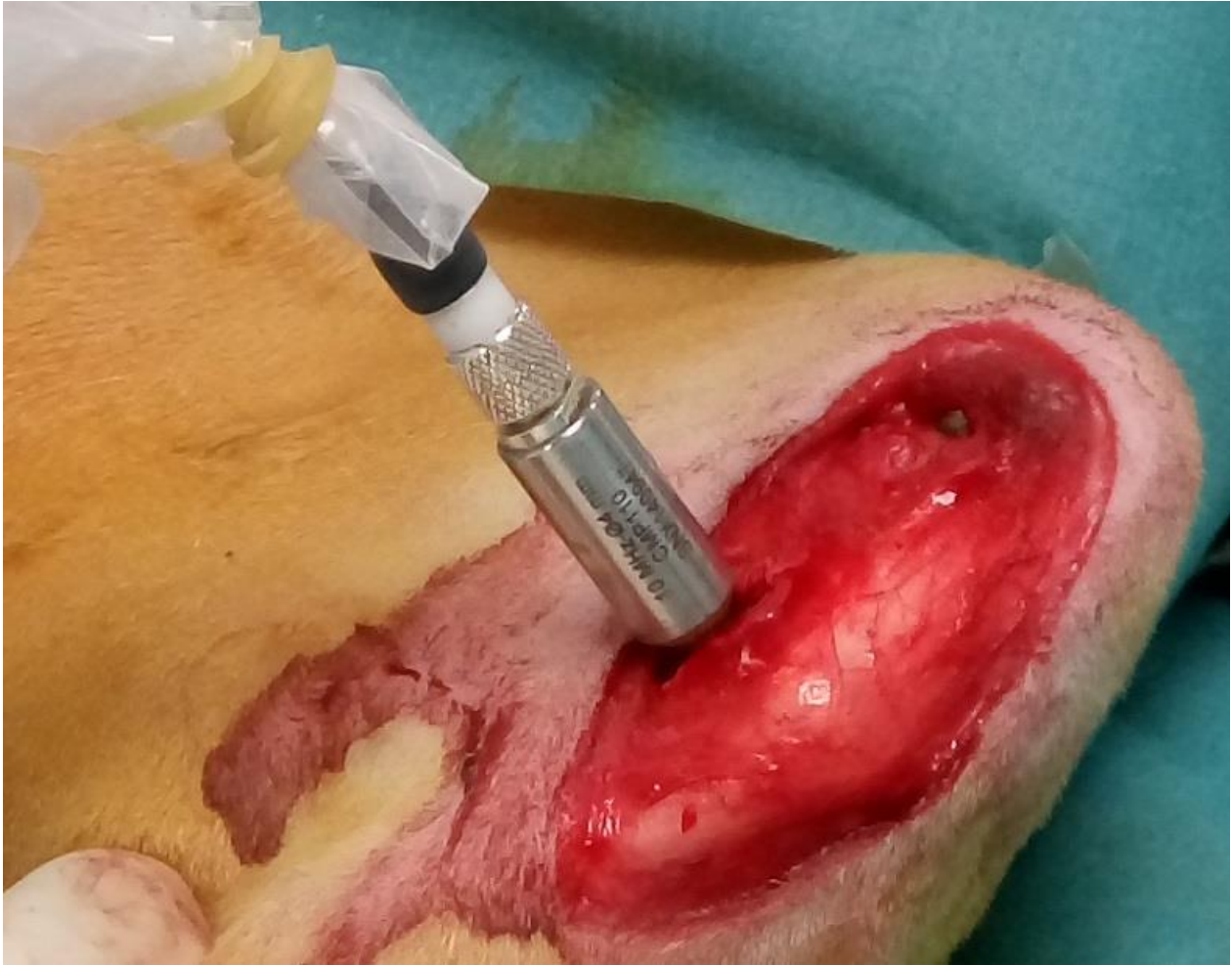
3 Figure 3: Measurement configuration of the ultrasonic indicator using the ultrasonic transducer screwed into 4 a dental implant.
