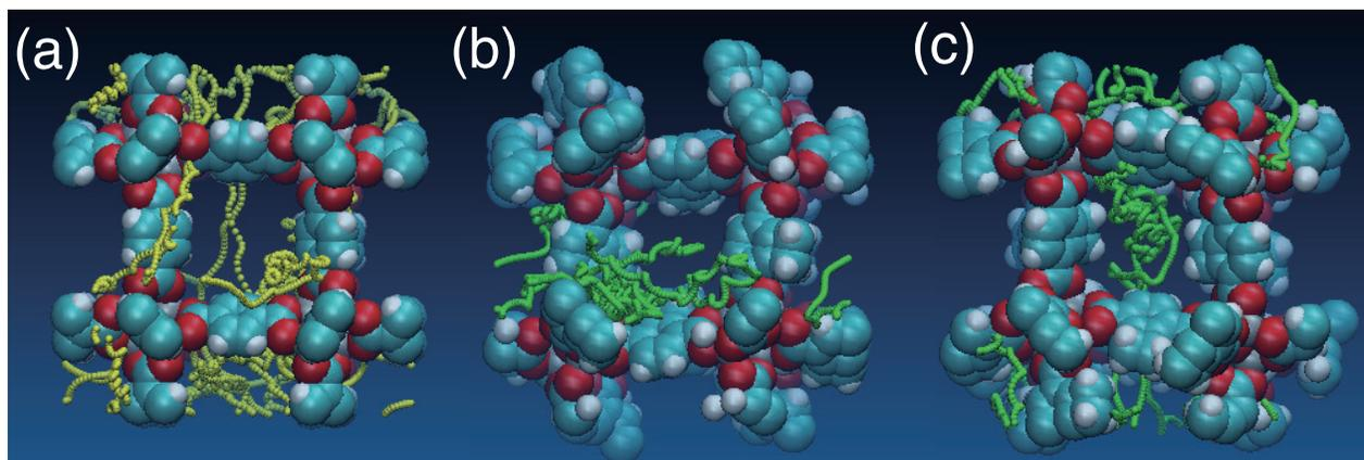
Figure 9: Trajectory of hydrogen molecules inside MOF-5 represented as a sequence of small yellow spheres (a) and inside IRMOF-6 in panels (b) and (c), each one referring to a different  $H_2$  molecule and represented as a sequence of small green spheres. The trajectories of the molecules are in each case subject to periodic boundary conditions and have not to be interpreted as broken on the cell borders. The color code for atoms is identical to what has been used in Figure 1.
