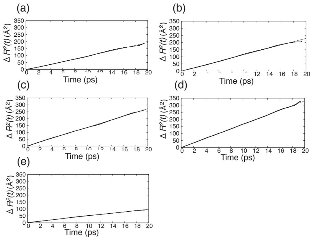
Figure 2: Mean squared displacements for the diffusions of  $\text{H}_2$  molecules inside the MOF-5 system at 200 (a), 300 (b), 400 (c) and 500 K (d), respectively. Panel (e) show the analogous mean squared displacement for IRMOF-6 at 200 K. The straight thin lines show the linear least square fitting and the thicker black lines the actual values computed from the displacement of the centers of mass of each hydrogen molecule.
