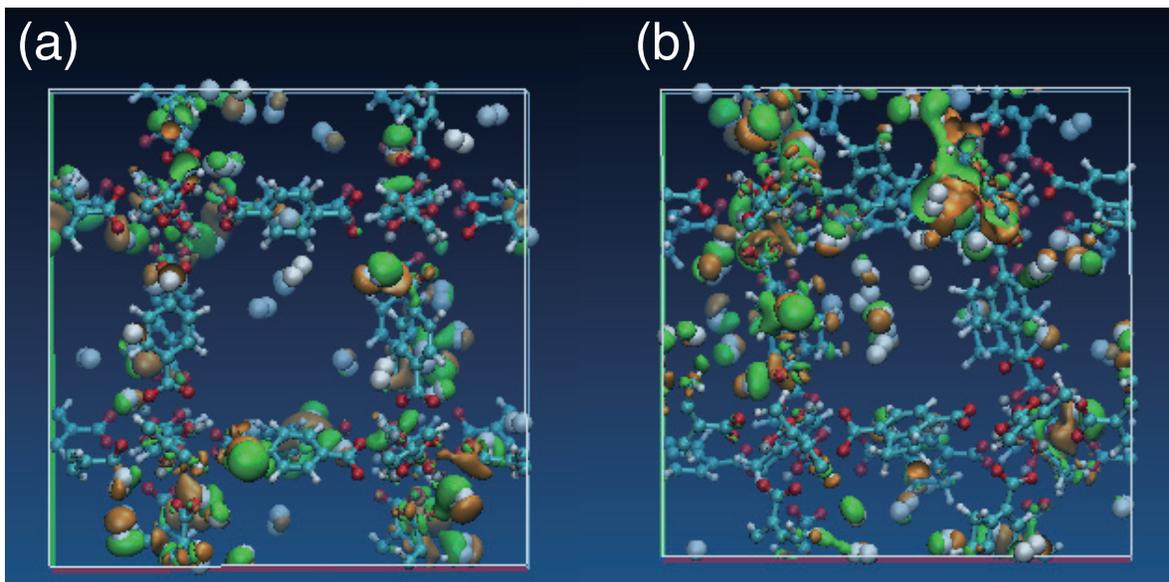
Figure 8: Charge density differences for MOF-5 (a) and IRMOF-6 (b). Green and orange colors indicate an increase and a decrease of charge density, respectively. Isosurfaces are shown at a value of  $\pm 1.0 \times 10^{-4} e/\text{\AA}^3$ . The color code for atoms is identical to the one used in Figure 1.
