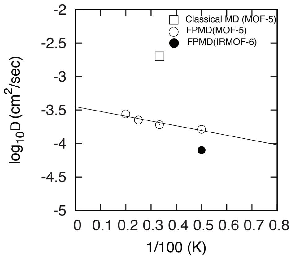
Figure 3: Diffusion coefficient of hydrogen molecules inside MOF-5 and IRMOF-6. The classical molecular dynamics result reported is taken from Ref.<sup>44</sup>
