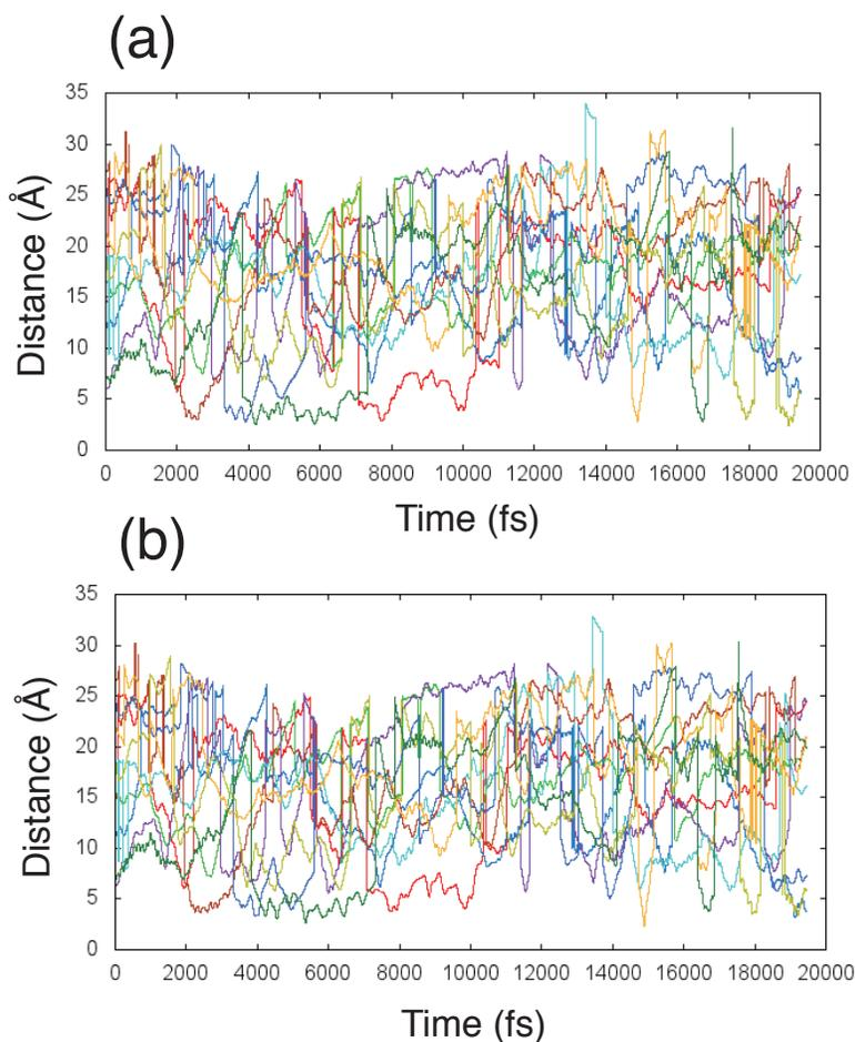
Figure 6: Distances of ten representative H<sub>2</sub> molecules from the Zn (a) and O (b) atoms belonging to a metal junction site. The Zn and O atoms are located in neighboring positions.
