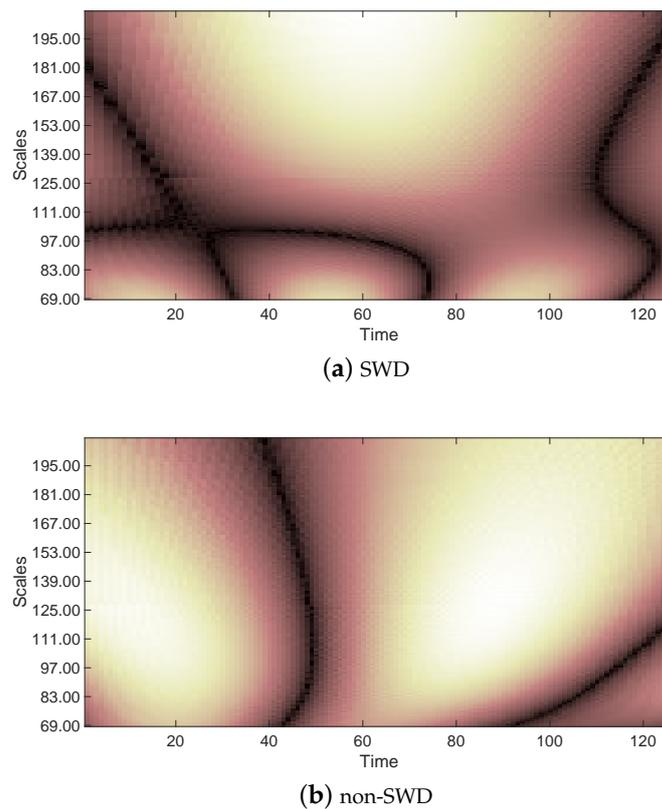
**Figure 3.** Illustration of the variation of time-scale for Morlet continuous wavelet (a) for SWD with  $f_c = 1.2308$  Hz, and (b) for non-SWD with  $f_c = 0.8125$ . Note that, the energy distribution pattern is different when comparing SWD and non-SWD.
