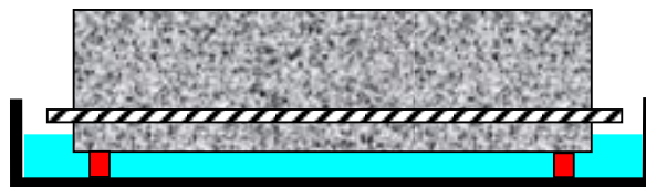
Figure 3. Scheme of the slab during the imbibition process in a pool filled with saline solution and showing the steel reinforcement.
