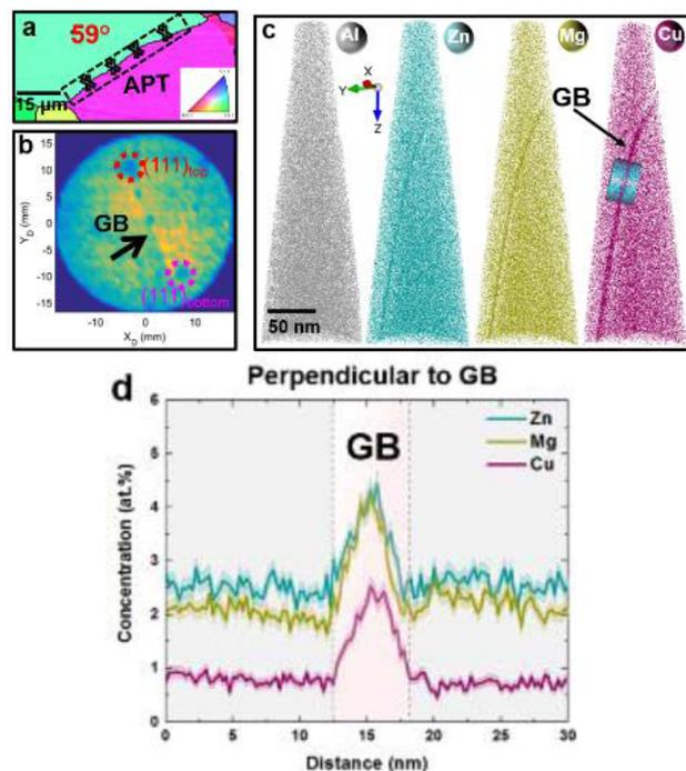
**Fig. 4.** APT analysis of the as-quenched Al-Zn-Mg-Cu alloy: (a) EBSD map showing the GB where APT tips were prepared; (b) Density map showing indexed crystallographic poles of the top and bottom grains; (c) Atom maps of all elements; (d) Composition profile across the GB.
