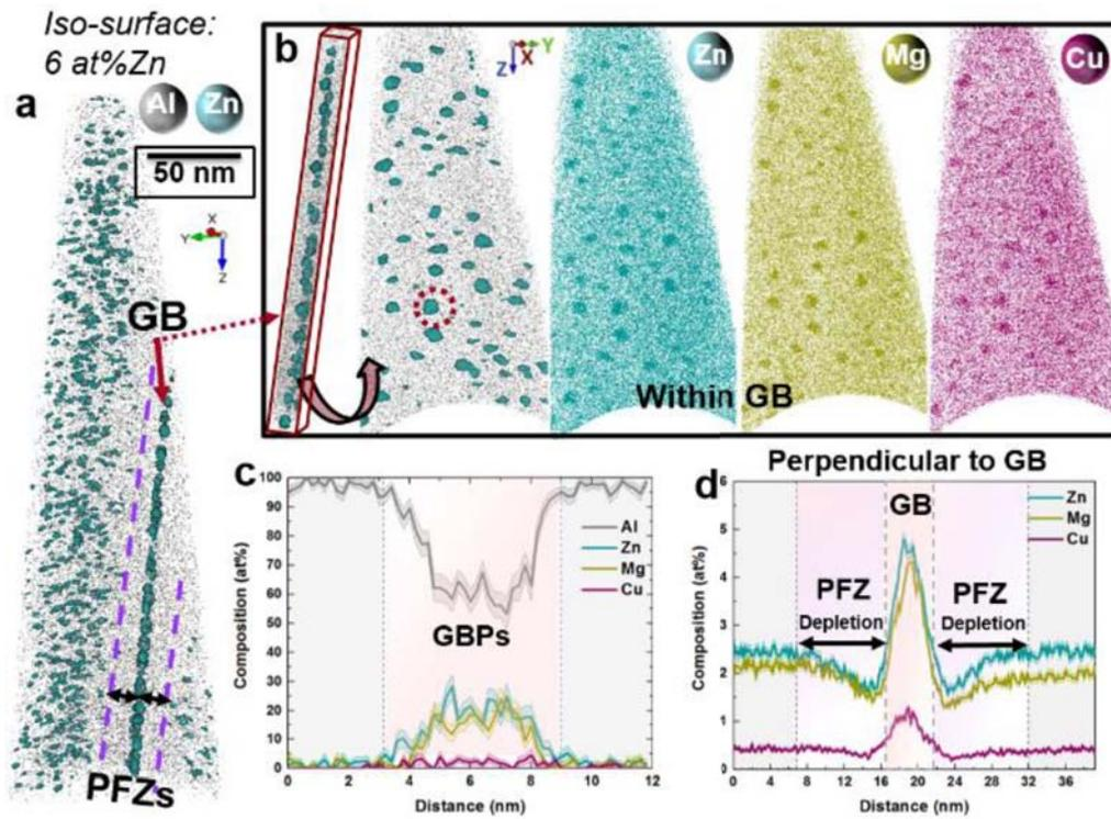
**Fig. 5.** APT analysis after aging for 0.5 hours at 120°C. (a) Precipitates visualized by iso-composition surfaces of 6 at% Zn; (b) Distribution of solutes along the GB plane; (c) 1D composition profile of the selected GB precipitate as indicated by the red circle; (d) 1D composition profile across the GB, devoid of GB precipitates. (Reprinted with permission from Ref. 37).
