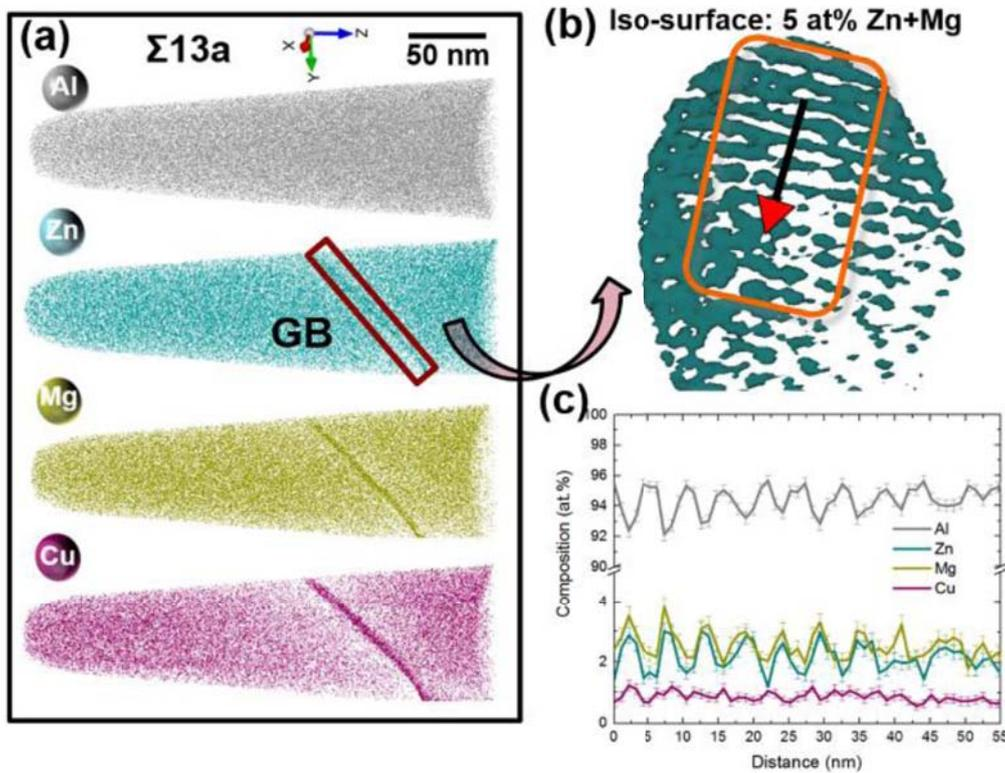
**Fig. 6.** (a) Atom maps of all elements of a  $\Sigma 13a$   $\langle 110 \rangle$  GB in the as-quenched Al-Zn-Mg-Cu alloy; (b) Distribution of solutes within the GB plane (region indicated by the red rectangle in (a)); (c) Corresponding one-dimensional composition profile along the arrow in (b). (The Figure was reproduced from Ref. 40, for which is under the terms of the CC-Attribution 4.0 international license)
