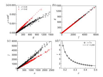
FIG. 17. (a) Relation between the density of mobile dislocations  $\rho$  and avalanche energy *E* for representative disorders  $\delta = 0.30, 0.42$ ; (b) dependence of *E* on the total distance covered by dislocations during an avalanche  $\bar{l}$ ; (c) dependence of  $\bar{l}$  on the number of moving dislocations *n*; (d) internal length scale *l* as a function of disorder strength  $\delta$ .
