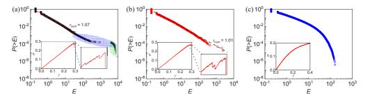
FIG. 11. Cumulative probability distributions of preyield avalanches at  $\delta = 0.28$  (a),  $\delta = 0.32$  (b),  $\delta = 0.7$  (c); to be compared with the data for 500 nm, 1000 nm, and 1500 nm Mo samples shown in Fig. 3(b). Averaging was performed over 100 realizations of disorder; insets show the stress-strain curves for a particular realization of disorder.
