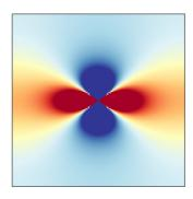
FIG. 5. The real-space representation of the dipole Fourier kernel  $\hat{L}(\mathbf{q})$ . Coloring: blue, negative; red, positive.
