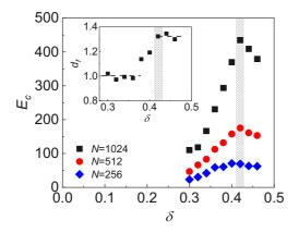
FIG. 13. The divergence of the cutoff size in the preyield regime around the critical value of disorder  $\delta \sim 0.42$ . Inset shows the behavior of the fractal dimension  $d_f$ ; the gray strip schematically marks the BD transition.
