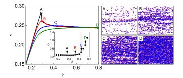
FIG. 7. The effect of disorder on the average strain-stress curves in simple shear tests. Inset shows the yield strain  $\gamma_y$  the gray strip schematically marks the BD transition. The zoom on the "after-yield" dislocation configurations is shown in the right column where the total number of dislocations is 782 (in A), 2600 (in B), 5220 (in C), and 8862 (in D). The dislocations with positive and negative Burgers vector are marked by red and blue. Parameters: K = 2, N = 1024.
