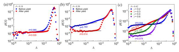
FIG. 16. Distribution of stability measures  $p(\Delta)$  at (a)  $\delta = 0.18$  (weak disorder), (b)  $\delta = 0.30$  (intermediate disorder) and (c)  $\delta = 0.42$  (critical disorder). In panel (c) we effectively show the function of two variables  $p(\Delta; \gamma)$ .
