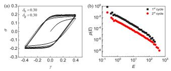
FIG. 23. (a) Strain-stress curves for the crystals subjected to six loading unloading cycles. (b) Avalanche distributions of cyclically loaded crystals for the first and the second cycles; the first cycle is understood as the monotone loading path. Here  $\delta_h = \delta = 0.30$ ,  $\delta_g = 0.30$ .
