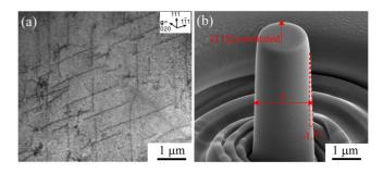
FIG. 1. (a) TEM image showing the grown-in dislocations in the bulk Mo crystal. (b) SEM image of [112]-orientated micropillar before compression.
