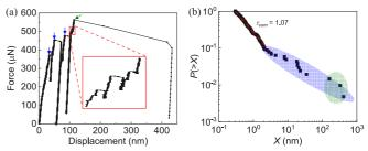
FIG. 4. Representative force-plastic displacement curve (a) and cumulative probability distribution of plastic displacements X detected over the entire deformation path (b) for the Mo pillars with 500 nm diameter.
