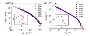
FIG. 14. Scaling collapse for the two cases: (a)  $\delta = 0.30$  (tuned spinodal criticality) and (b)  $\delta = 0.46$  (BD criticality). Insets show schematic stress-strain curves around spinodal *S* and critical *C* points.
