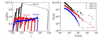
FIG. 3. Compression tests on pure Mo submicron pillars: (a) stress-strain curves (shear); (b) cumulative distribution of plastic displacements X detected over the entire loading process. Here  $\tau_{cum} = \tau_{in} - 1$  where  $\tau_{in}$  is the stress-integrated exponent.
