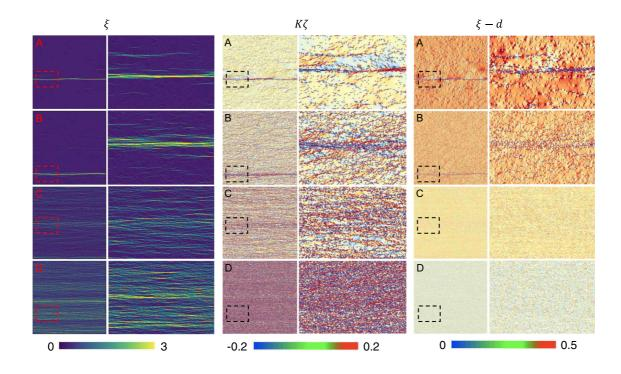
FIG. 8. After-yield spatial patterns: shear strain  $\xi$ , longitudinal stress  $\sigma_{xx} = df/d\zeta = K\zeta$ , and shear stress  $\sigma_{xy} = df/\xi = \xi - d$  in the reference coordinates. Strength of disorder:  $\delta = 0.28$  (A),  $\delta = 0.36$  (B),  $\delta = 0.42$  (C) and  $\delta = 0.46$  (D). Zoomed views of the marked areas are shown in parallel columns.
