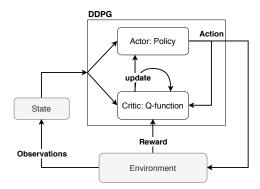
Fig. 4: Overview diagram of the DDPG algorithm
