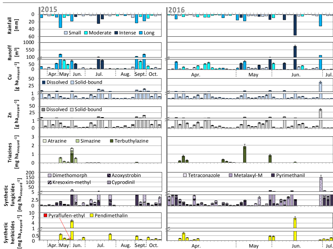
Figure 3. Rainfall, discharge and normalized loads of Cu, Zn and synthetic pesticides exported from the vineyard catchment (Rouffach, France; 25.3 hectares of vineyards). 32 and 46 events were monitored in 2015 and 2016, respectively. The error given for discharge measurements corresponds to the measurement precision (8%). The errors given for the pesticide loads were calculated via error propagation and incorporate errors associated with discharge measurements and pesticide quantification (see Table S2).
