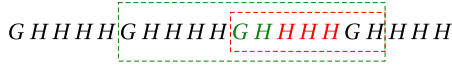
FIG. 9. Diamond chain where only hub sites a are represented by the letter H (for Hadamard) or G (for Grover) standing for the coin used on the hub site. In between hub sites, composite shift operators K = S \cdot U_2 \cdot S are always present but not represented. Dashed red (resp. green) box delimits the extension of the cage for an initial state on red (resp. green) sites at flux 1/2 .
