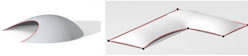
Figure 14 Examples of LW surfaces bordered by funicular arches
